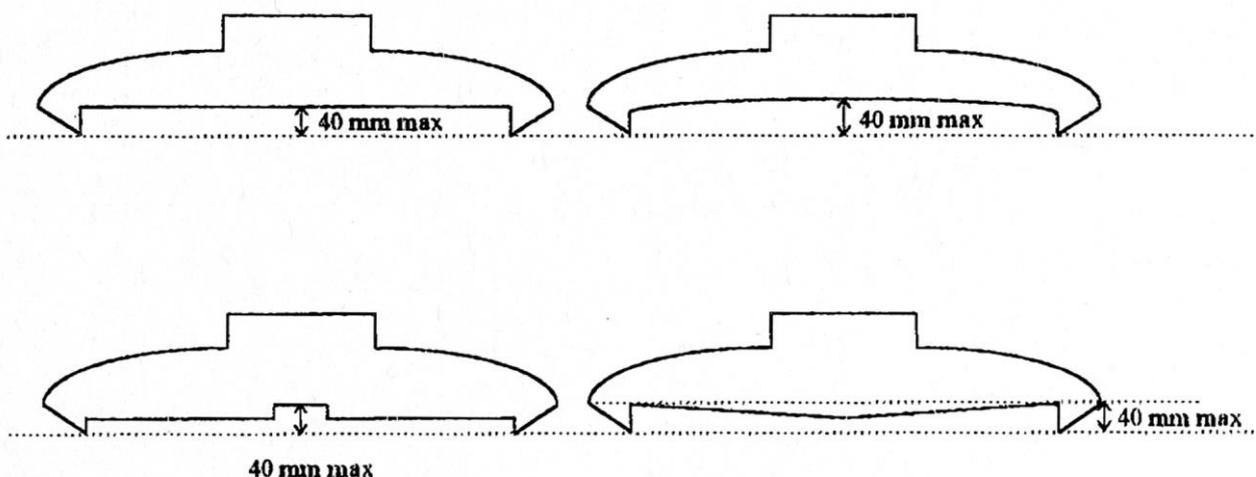
For the classes F500 and F700, hull type must be a catamaran type, based on twin hulls, but may be of completely free hydrodynamic and aerodynamic design.
