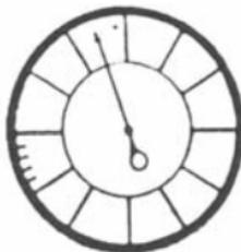
This clock is to be driven electrically or mechanically. It has only one hand moving continuously and indicating the seconds.
