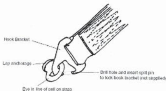
A split pin must lock the seat belt hook to the lap anchorage.
