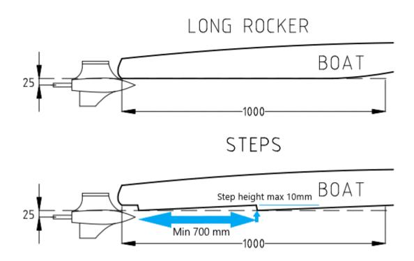
HYDROPLANE AND OSY400 PROPELLER SHAFT HEIGHT MEASUREMENTS
