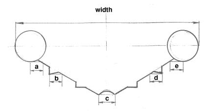
For PR 550, 700, 750, 850 : a+b+c+d+e < 10 % of the width For PR 1000, 1500, 2000, 3000 : b+c+d < 20 % of the width
