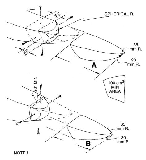
PICKLEFORK MUST DEFORM AT 100 kg MAXIMUM
