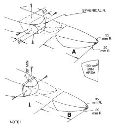
PICKLEFORK MUST DEFORM AT 100 kg MAXIMUM
