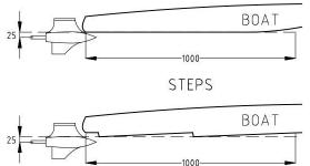
HYDROPLANE PROPELLER SHAFT HEIGHT MEASUREMENTS
